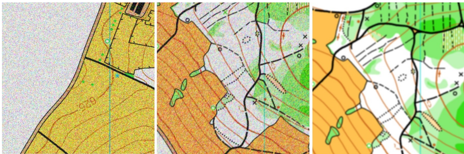
Figure 1. Examples of augmented training tiles used for contour segmentation. The augmentations increase appearance variability while preserving the geometric consistency of the contour labels.
