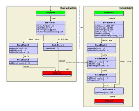
Figure 2: Control flow graph of the sample code shown in Listing 1
